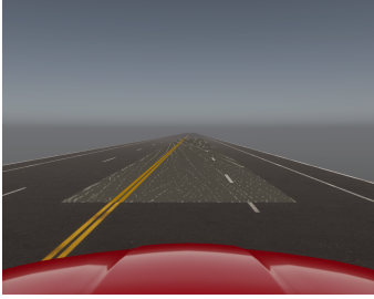
Fig. 2: Image of the adversarial patch captured by front camera.
