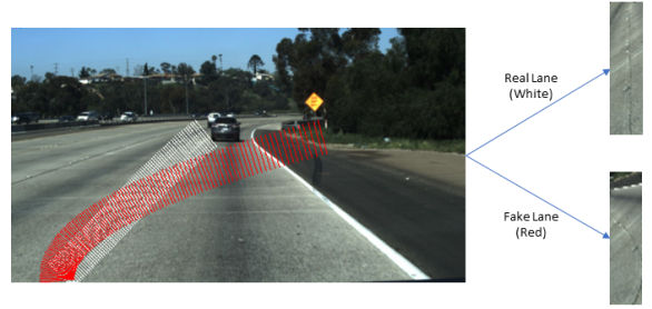
Fig. 4. Examples of positive and negative examples generated by the lane stabilization process for the defense training dataset.
