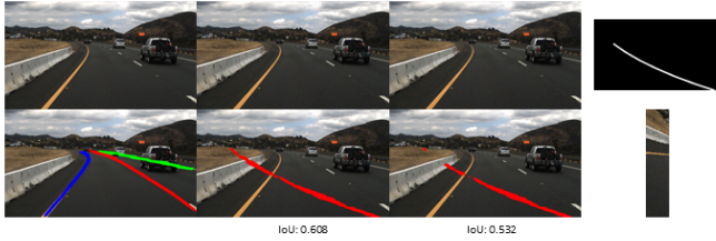
Fig. 5. Example of L-infinity bounded attack. From left to right, the vertical pairs of images represent clean, nonadaptive, and adaptive attack, with the lane detection model output superimposed on the second row, and IoU values below. IoU values are with respect to the upper rightmost image of the target lane binary segmentation map, and the resulting stabilized lane is shown below. Under bounded attack, the attacker is able to assert full control over the scene and induce arbitrary lane configurations.
