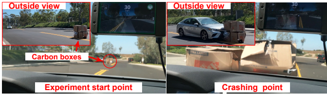
Fig. 4: Safety impact evaluation for our attack on a Toyota 2019 Camry with OpenPilot engaged. Even with other driver assistance features such as Automatic Emergency Braking (AEB), our attack still causes collisions in all the 10 trials.
