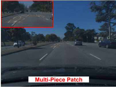
Fig. 1: Driver’s view in multi-piece patch attack mode (§II) at 2.5 seconds before the attack succeeds. The attack in the figure has 8 pieces of 1.8\text{m}\times 7.2\text{m} road patches, each requiring only 5-10 sec to deploy for 1-2 people.
