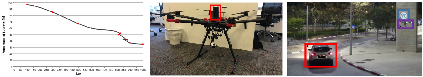
Fig. 4. Left: Influence of Ambient Light. Middle: the drone with the projector used in our experiments, Right: the moment of the attack (the projected road sign is boxed in blue, the attacker’s drone is boxed in purple, and the victim’s car is boxed in red).
