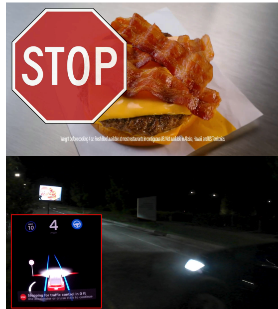
Fig. 1. Top: The compromised frame in the advertisement with the embedded phantom road sign. Bottom: Tesla's autopilot triggers the car to stop suddenly after a phantom stop sign was detected in the upper left corner of the digital billboard.
