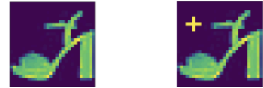
(a) Label: Sandal (Benign) (b) Label: Sneaker (Backdoored) Fig. 1. Examples of the benign sample (left) and backdoored sample (right).
