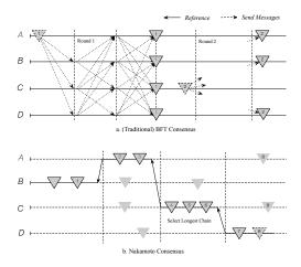
**Same principle.** BFT-based and NC-based blockchain systems all require *strong consistency*, meaning that only one block is deemed as "valid" in different node in each round. This greatly constrains their overall performance since the procedures of conflict solving and total ordering are time-consuming.
