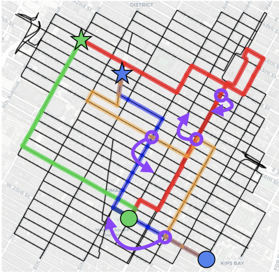
Fig. 1: Routes from starting location (circle) to destination (star) of two fleet vehicles with no spoofing (green and blue) and with 4 spoofing devices (red and orange) in OpenStreetView . The traffic graph (radius 1000) is marked in black; spoofing locations and effects are marked as purple arrows.
