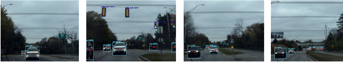
Fig. 9: Tracking the following vehicles over the continuous time frames. Each figure shows the detected following vehicles at the rear view of our vehicle.
