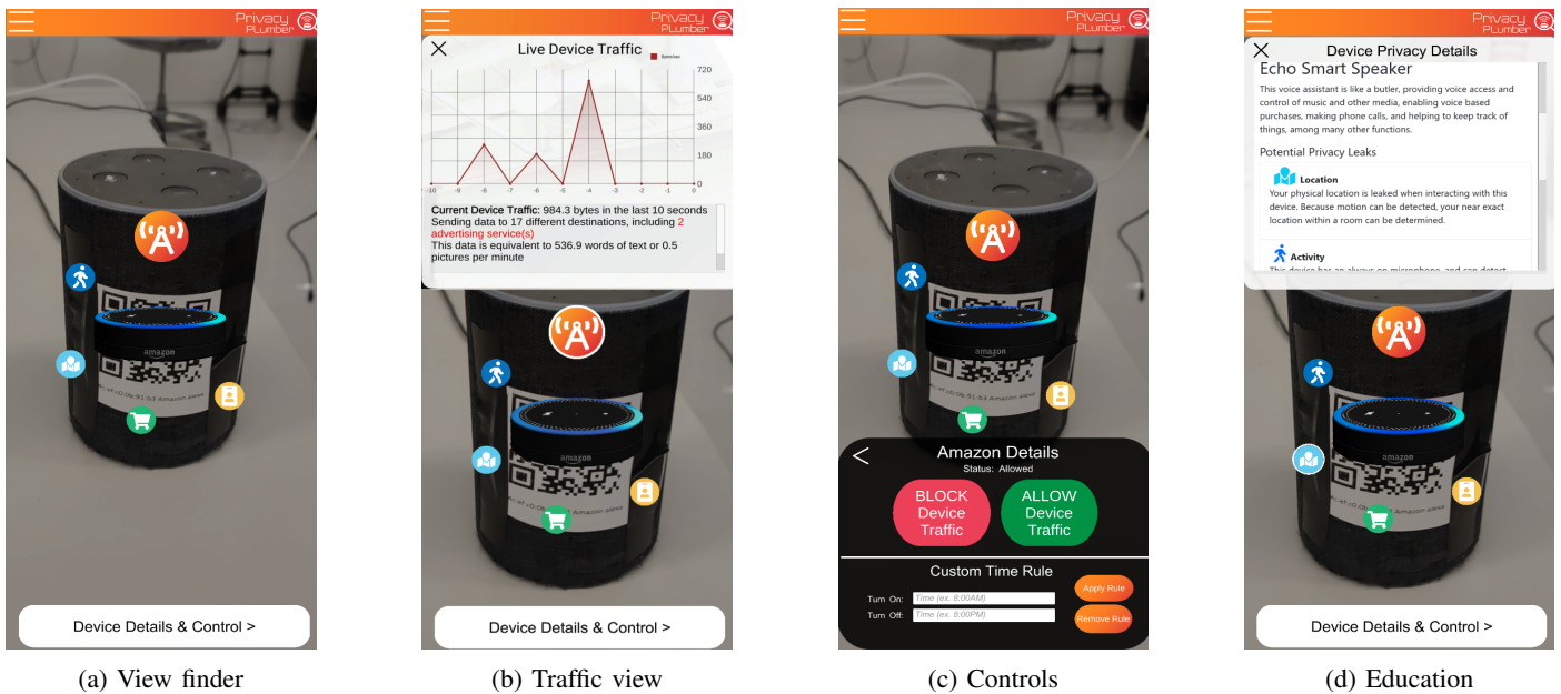
Fig. 4: Illustration of mobile application design. (a) Device recognition with interactive menu. (b) Live traffic inspection. (c) Rule-based device traffic control (i.e., blocking and unblocking). (d) Educational material on privacy details.
