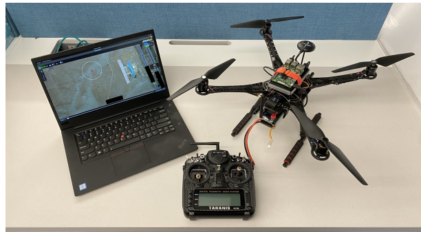
Figure 4: Hardware setup showcasing the Holybro S500 drone, the radio controller, and the ground control station.
