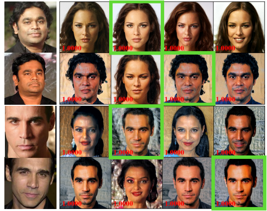
Fig. 10: Effects of dropout and consistent selection strategy. The first column shows two images of each target person. The odd/even row shows the inversion results without/with dropout strategy. The final images selected by our consistent selection strategy are highlighted by green squares. Numbers denote the target confidence.
