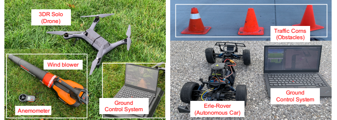
Fig. 9: Real vehicles and experimental tools. Aerial vehicle setup (left): drone, GCS, wind generator, and anemometer. Ground vehicle setup (right): traffic cones, GCS, and autonomous vehicle.
