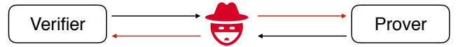
Fig. 2. In Mafia Fraud, an external attacker reduces the distance measured between two mutually trusted parties.
