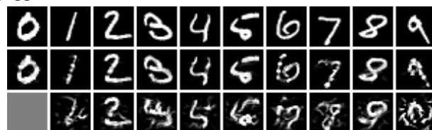
Fig. 10: Adversarial Samples. 1st line shows seed inputs, 2nd line shows without detector, 3rd line shows with 1 detector. Gray boxes mean no adversarial samples found in 1000 iterations.
