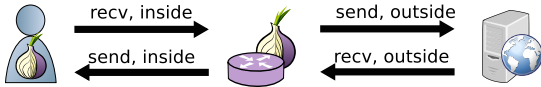
Fig. 5. A relay may send and receive a different number of cell types on the inside and outside of a circuit.
