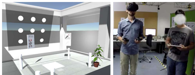
Fig. 1: We investigate how to create seamless and secure authentication in VR. In particular, we compare different screen sizes, input modalities, and password types with regard to how secure they are against attackers in the real world. The left image shows a sample view of a [virtual] large display supporting lock pattern input in VR. The right image shows a user in the real world, authenticating in this environment whilst being observed by an attacker. The user is wearing a head mounted display (HMD) and holding one controller in each hand to enable interaction in VR.
