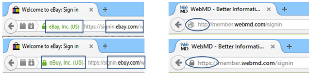
Fig. 2. Example website manipulations. On the left a sample eBay spoof (Bottom) compared with the legitimate eBay site (Top). On the right a login site with the encryption removed (Top) compared to the legitimate site with a standard certificate and encryption (Bottom).
