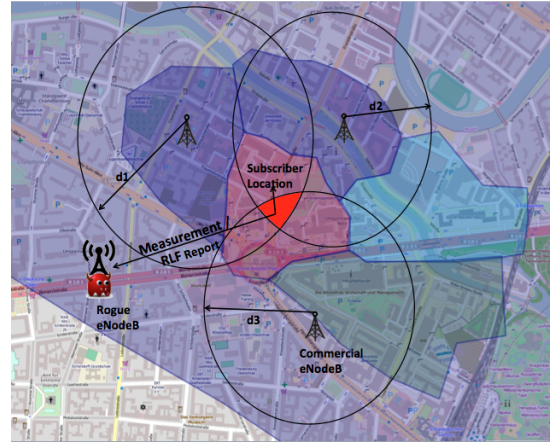
Fig. 7. Determining subscriber’s precise location using trilateration (L3)
