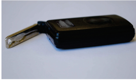
(a) A PKES Key and its backup physical key.
