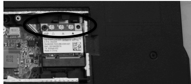
Type 1: internal antennas for Dell E5400 laptop
