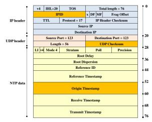
Fig. 1. Mode 4 NTP Packet, highlighting nonces and checksums.
