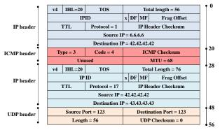
Fig. 3. ICMP Fragmentation Needed packet from attacker 6.6.6.6 telling server 42.42.42 to fragment NTP packets for client 43.43.43.43 to MTU of 68 bytes.
