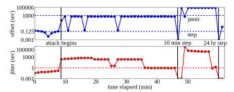
Fig. 6. Absolute value of offset  $\theta$  (above) and jitter  $\psi$  (below) computed by the client during a proof-of-concept implementation of our attack.
