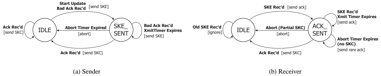
Figure 4. Simplified state diagrams for the (a) sender and (b) receiver of a reliable key update.
