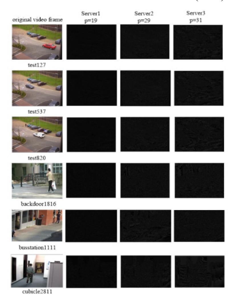
**Encrypted video frames** The original frames are split into encrypted shares. The video contents are protected and nearly nothing can be recognized in the cloud servers.
