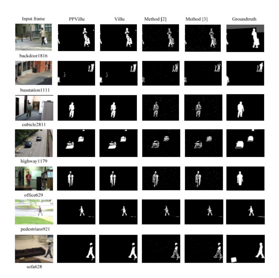
**Background Extraction Results** We get the same background using ViBe by multiple cloud servers from encrypted frames or unencrypted frames. Thus the results from ViBe background extraction are the same, whether video frames have been encrypted or not. Furthermore, the information of video frames will not directly exposed in cloud servers after be encrypted. This strategy is an efficient way to protect the privacy of user videos.
