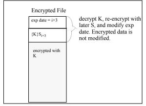
Figure 2. Delaying a file's expiration: encrypting data with file key K, encrypting K with S<sub>i</sub>
