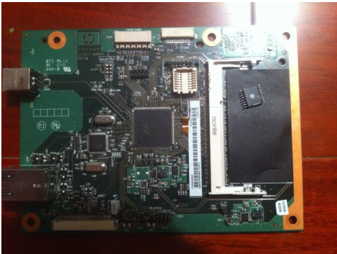
Fig. 2. Formatter board for LaserJet P2055DN. Dump of the onboard SPI flash revealed RFU format and integrity checking algorithm.
