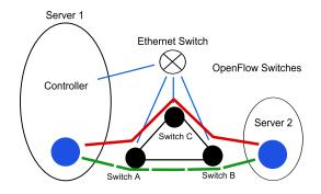
Fig. 6. Our evaluation setup. All OpenFlow switches are connected to each other on the data plane, and connect to the controller in a star topology via an Ethernet switch. We assume that user-defined path setup between "Server1" and "Server2".
