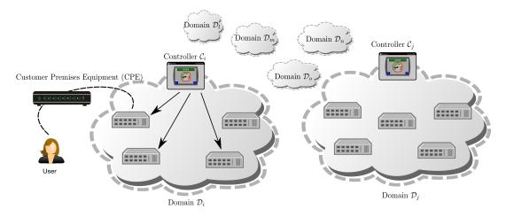
Fig. 1. System model. We assume a network comprising of one or more OpenFlow-supported domains. Each domain  $D_i$  is governed by a (logically centralized) controller  $C_i$ . Users are connected to the network by means of CPEs.
